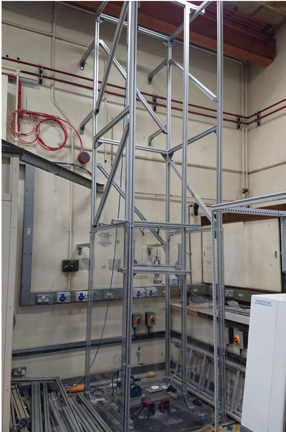
Figure 6. The rigid body drop tower with 4 meters drop capacity and all sides protected by polycarbonate sheets.
